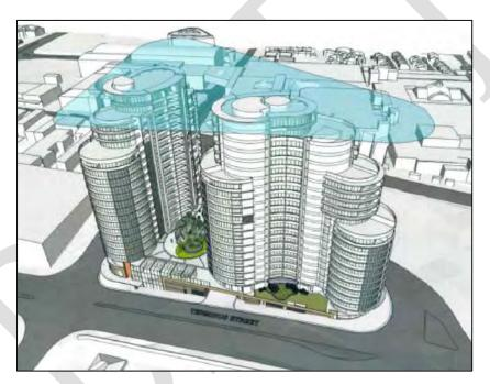
It is noted that the blue layer illustrates the 68 metre height plane measured from natural ground level. The proposed encroachments relate to the lift overrun and a portion of the roof parapet as illustrated in the figure above.
